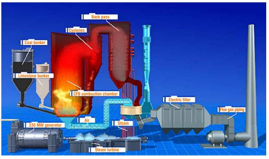
Fig. 43. Flowchart of a coal-fired generation unit at a State District Power Plant (GRES)
